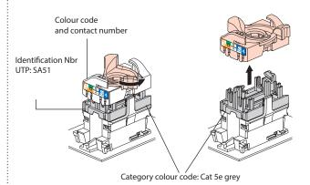
This system allows the wire pairs to be spread easily before mounting them on the connector.
