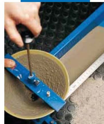
Test de curgere conform UNI 13395-2
