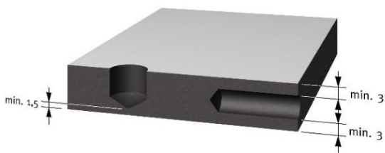
Figure 5: Minimum distances of the drill holes to the edge of the board
