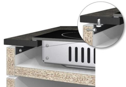
Figure 51: Stabilisation with metal traverse
