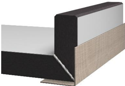
Figure 18: Fold up the upstand and secure with adhesive tape
