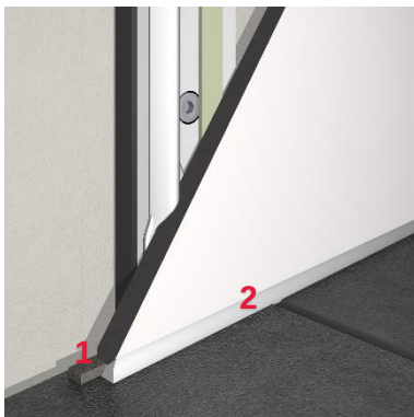
Figure 32: Flushfloor installation for shower area
