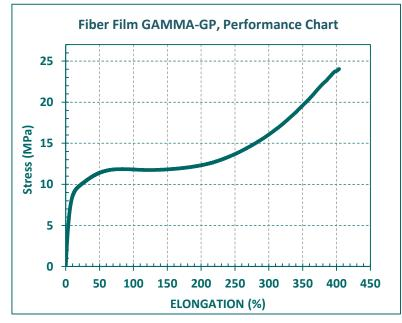
The graph above illustrates how the film performs under an increased load. Where the line ends indicates where the film breaks.
